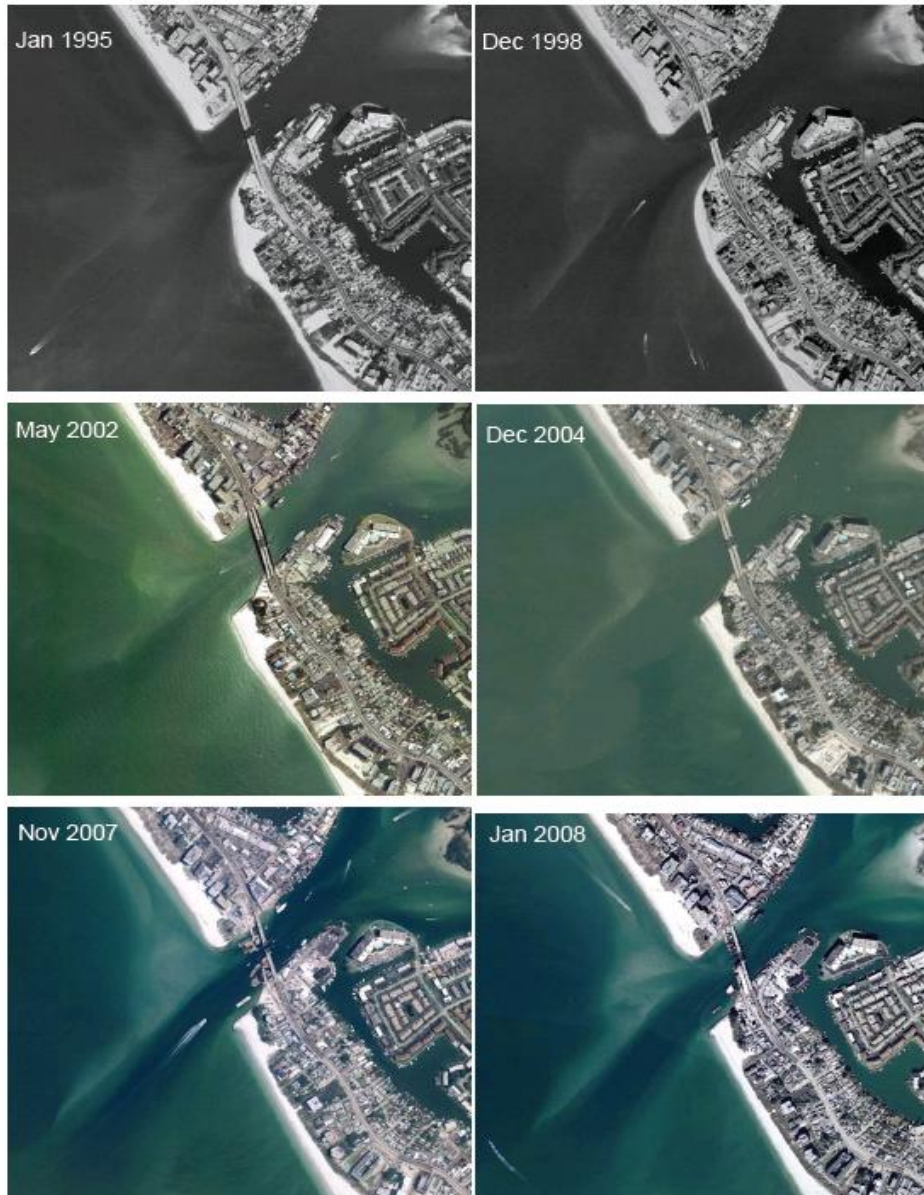
Figure II-73. Sequential Vertical Aerial Photographs of John's Inlet between 1995 and 2008 (from Google Earth)
