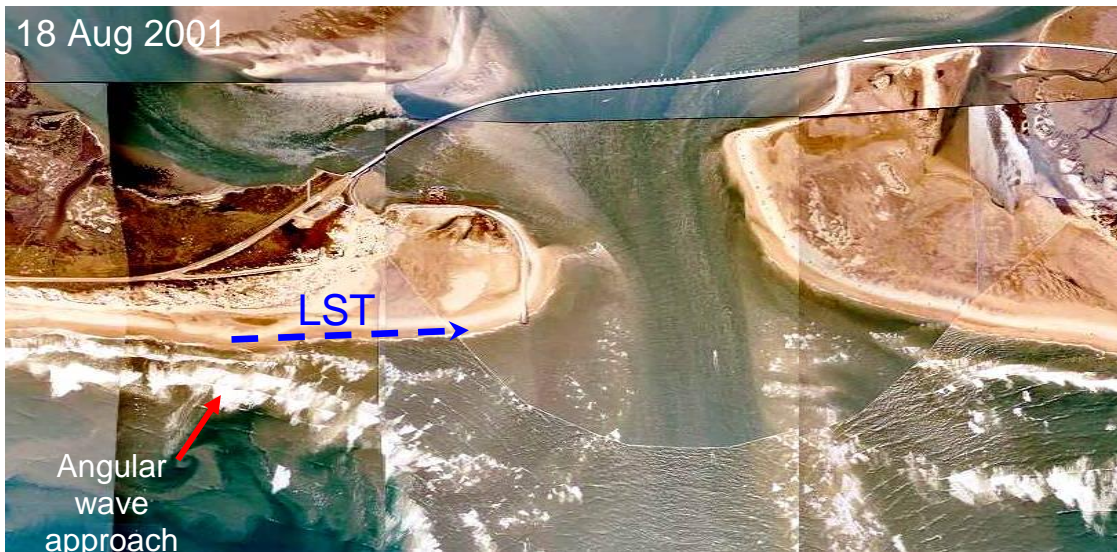
Figure II-12. 2001 Aerial Photograph of Oregon Inlet Showing Wave Refraction Around Ebb Delta Producing Northerly Transport Along Pea Island Feed Sand to the Fillet Region. Note the sand that has moved past the groin and constructed a beach along the inlet shore
