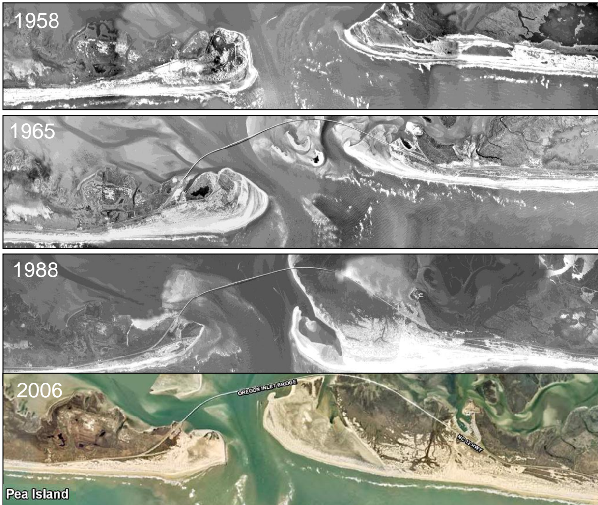
Figure II-13. Sequential Photographs of Oregon Inlet Depicting the Shoreline Changes Associated with Spit Accretion at Bodie Island and Southerly Migration of Oregon Inlet (Cleary, 2009)
