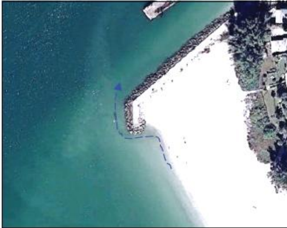
Figure II-72. Vertical Aerial Photograph of the Terminal Groin at the South Side of John's Pass at the Northern End of Treasure Island (from Google Earth)
