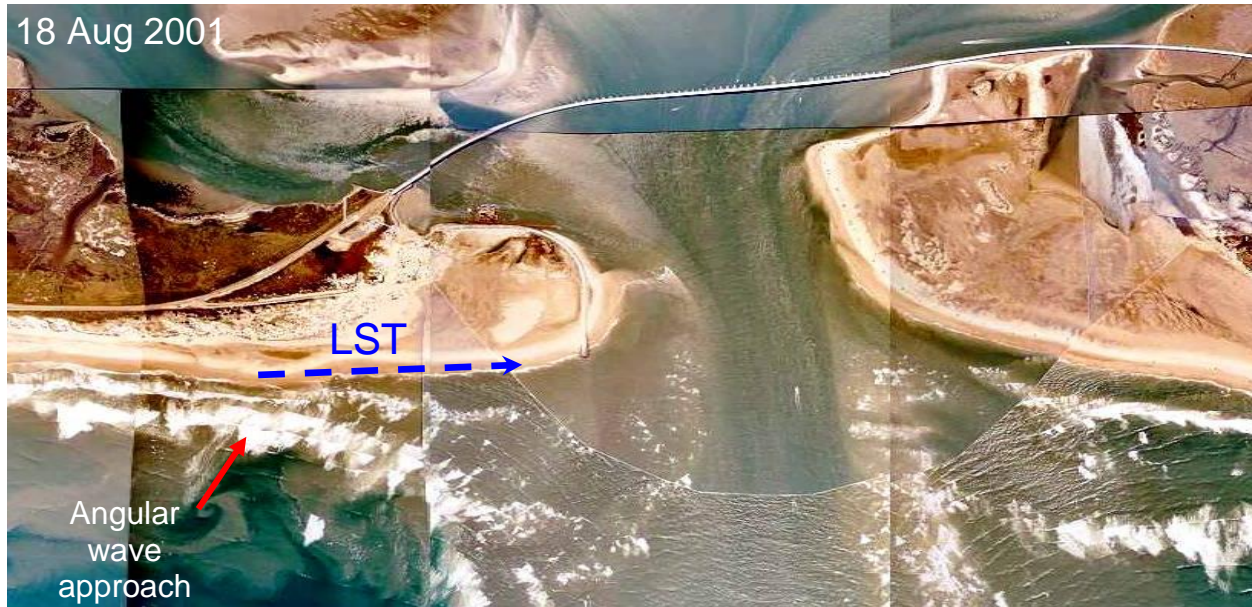
Figure III-9. 2001 Aerial Photograph of Oregon Inlet Showing Wave Refraction Around Ebb Delta Producing Northerly Transport Along Pea Island Feed Sand to the Fillet Region. Note the sand that has moved past the groin and constructed a beach along the inlet shore
