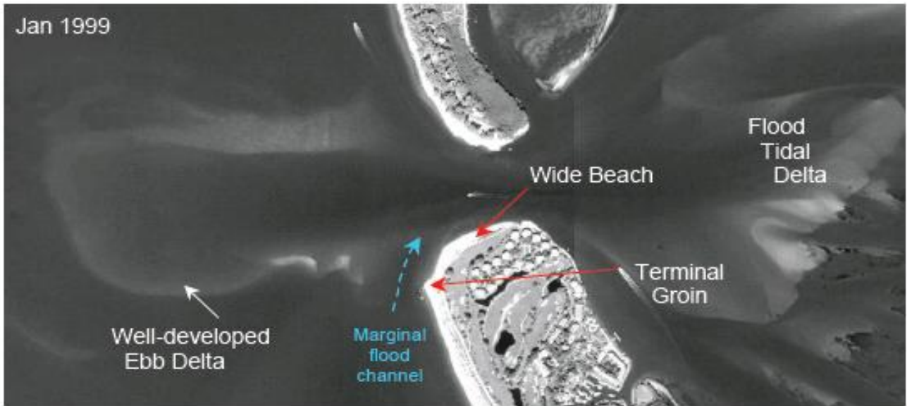
Figure III-34. View of the Ebb-tidal Delta That Has Been Used as a Source of Sand for Nourishing the Beach Along Captiva Island (from Google Earth)
