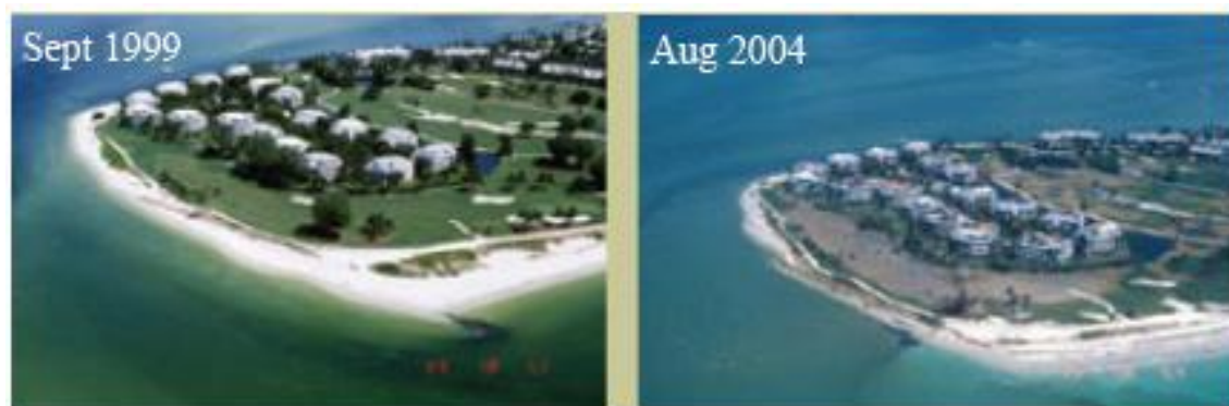
Figure III-38. Comparison of Photographs Taken Before and Immediately After the Passage of Hurricane Charley Showing Beach Erosion Inside the Inlet
