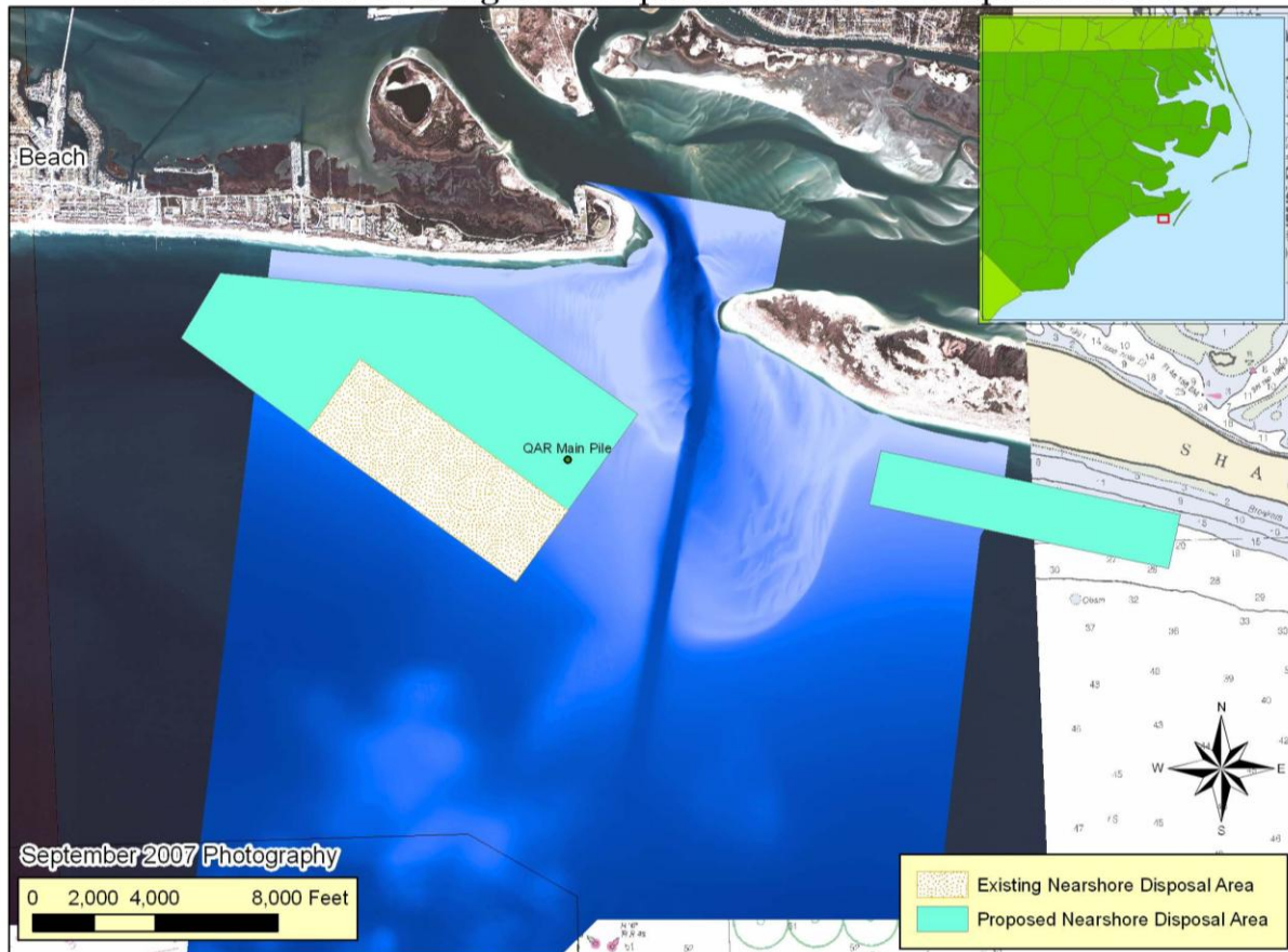
Figure IV-14. Existing and Proposed Nearshore Disposal Locations for Beaufort Inlet Source: USACE – Wilmington District (2009)
