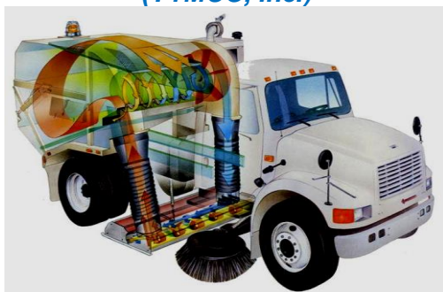
Figure 17. Regenerative Air Cleaner (TYMCO, Inc.)
