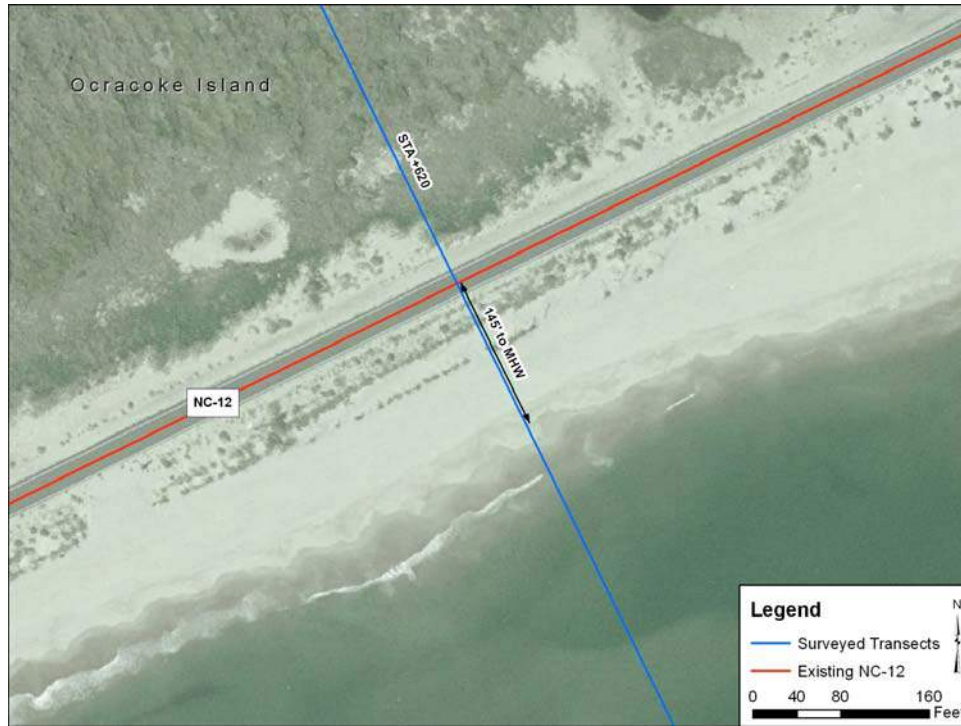
Figure 4. Plan View Illustrating Setback of Roadway Centerline from the MHW at station 620+00
