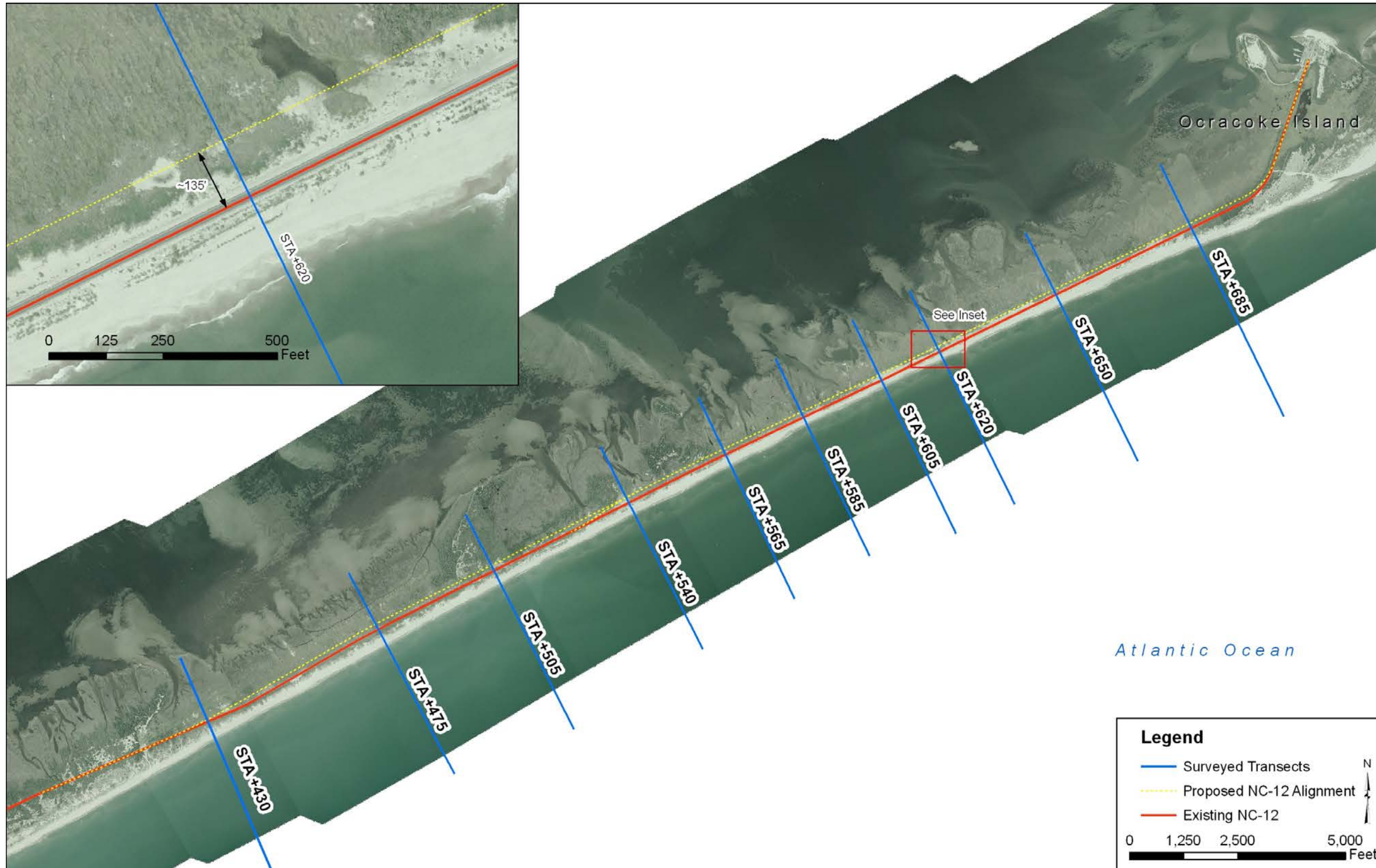
Figure 14. Proposed Roadway Realignment
