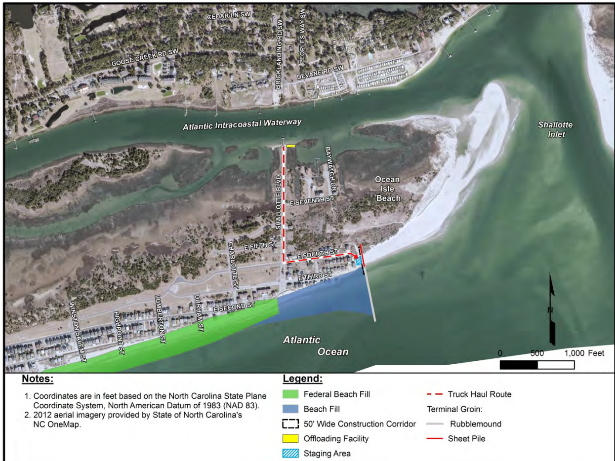
Figure 4. Location of the proposed terminal groin and associated beach fill located on the eastern portion of Ocean Isle Beach
