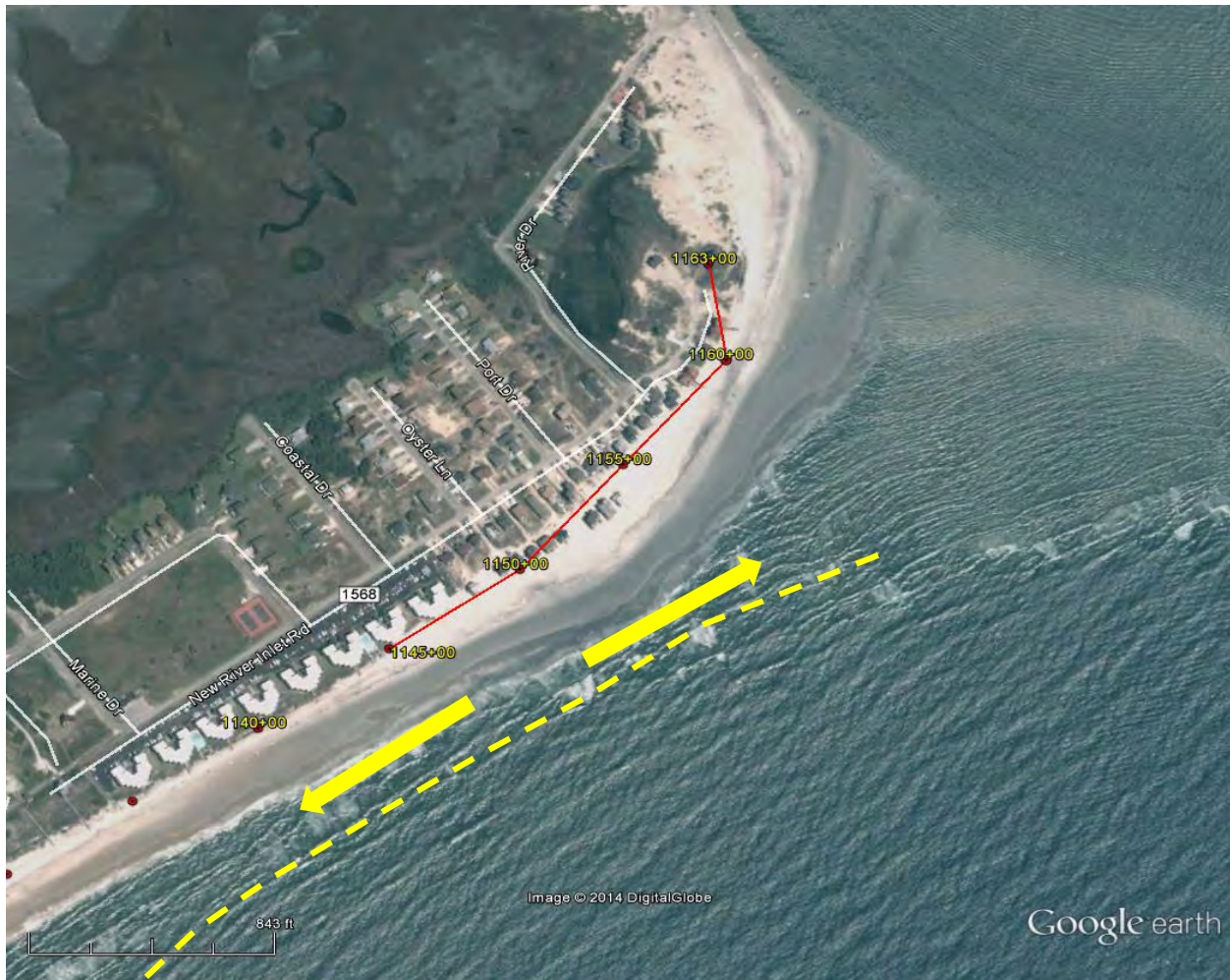
Figure 2. August 2002 Google Earth photo showing wave refraction patterns and direction of littoral sand transport just south of New River Inlet. Note: bulge in shoreline was due to disposal of navigation maintenance material removed from the AIWW by the USACE.
