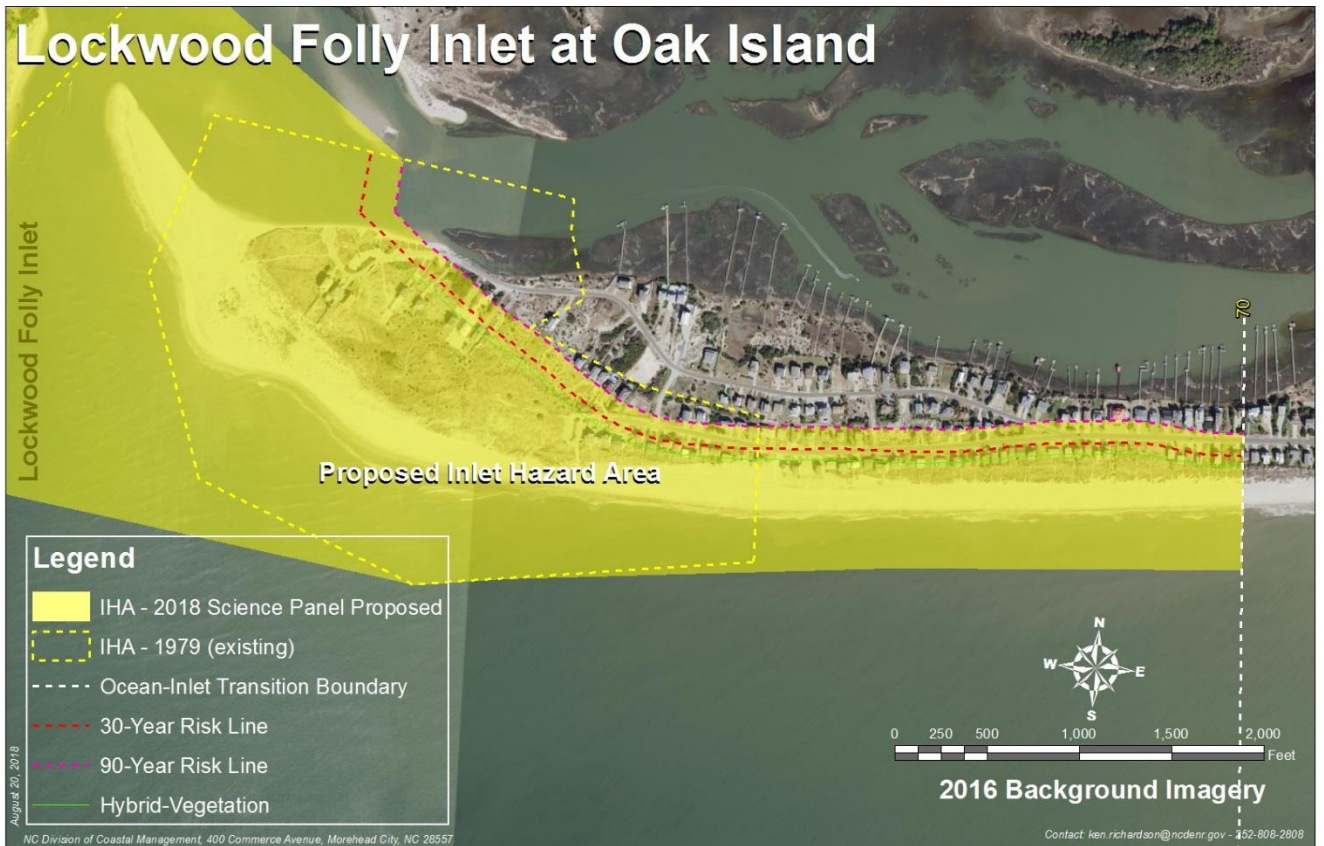
Figure 30. Lockwood Folly Inlet at Oak Island Hybrid Vegetation Line and the recommended IHA boundary with the 30- and 90-Year Risk Lines.
