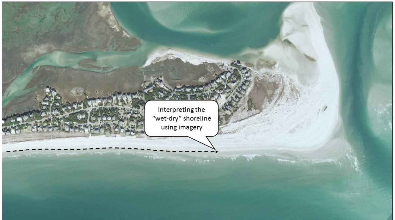
Figure 4. Interpretation of the "wet-dry" shoreline using orthophotography.
