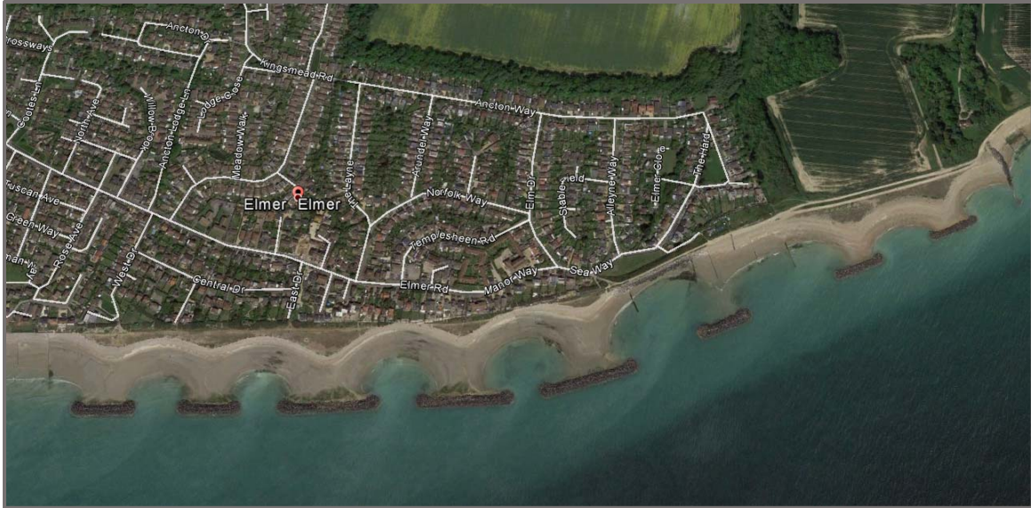
Figure 18. Breakwaters installed at Elmer, UK. Although erosion appears to be reduced, these structures do interfere with sediment transport causing a “scallop effect” on the beach as sediment fills in behind each breakwater.
