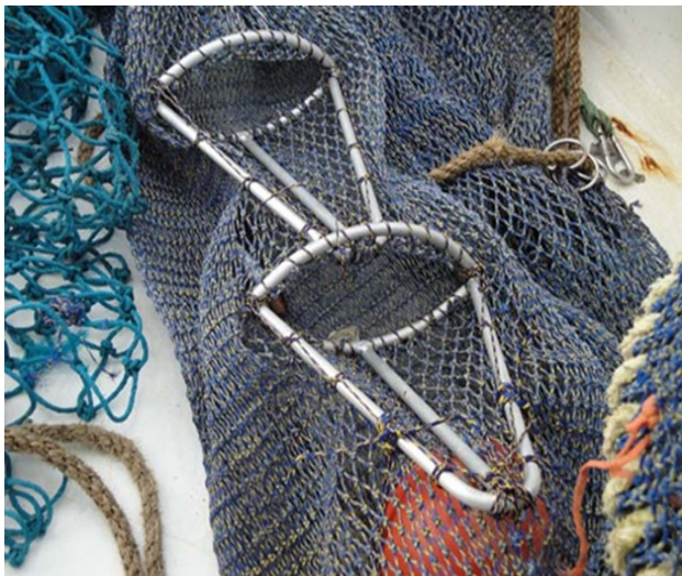
Examples of Industry Workgroup gear combinations that reduced bycatch by 40 to 57%
