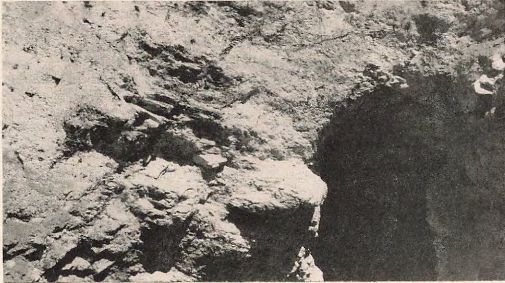
A. Steeply dipping quartz fracture fillings (to left of opening) cutting pegmatite at mouth of chamber, Carson mine, No. 3 working. The most prominent fracture filling is about 4 inches in maximum thickness.
