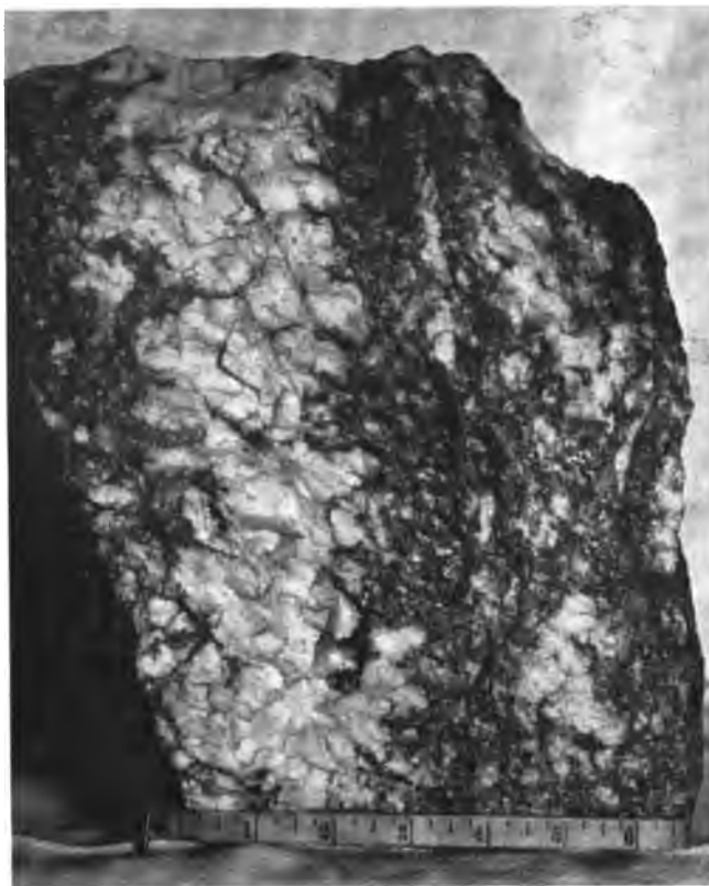
(A) Photograph of a specimen of ore from the Wall mine showing the relation of ore and gangue. The vein was divided at the point from which this specimen was taken, and the piece here figured represents the entire width of one portion of the vein. Dark areas = ore, chalcocite and bornite. Light areas = vein matter, largely quartz.
