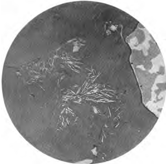
(A) Photograph, natural size, of a specimen of ore from the Copper King mine showing association of ore (chalcocite and bornite) and calcite. Some of the calcite which is imbedded in the sulphides is in the form of well-terminated crystals.
