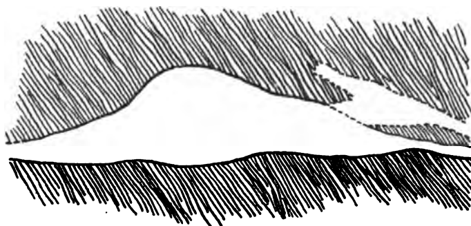
Fig. 12.—Sketch showing cross-section of the Holloway vein as seen in the 300-foot level, south. (After Weed.)
