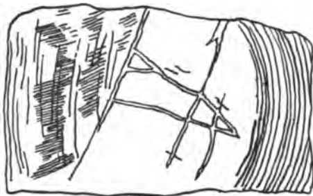
Fig. 10.—Sketch showing face of 300-foot level, south, in Holloway mine, January 26, 1900. On the left, black quartzose ore; in the center, white quartz stringers in black gangue. (After Weed.)
