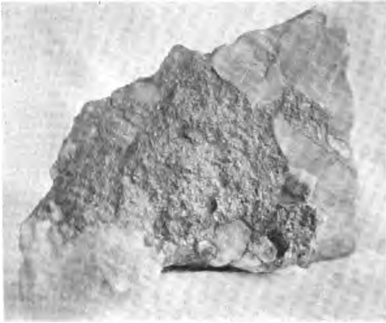
(A) Photograph, natural size, of a specimen of ore from the Copper King mine showing association of ore (chalcocite and bornite) and calcite. Some of the calcite which is imbedded in the sulphides is in the form of well-terminated crystals.
