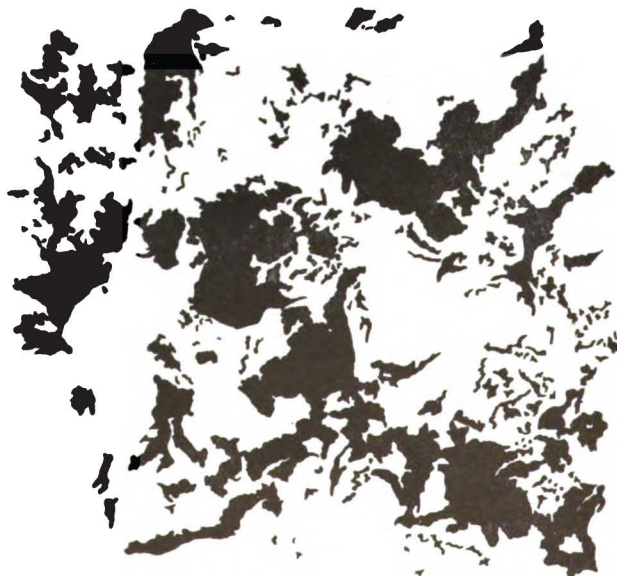
(B) Tracing made from a polished surface of a specimen of ore from the Wall mine, natural size. Shows the relation of the ore to the quartz gangue. This relationship is typical of all the mines in the district. The ore and quartz appear to be of contemporaneous deposition. Black = ore, chalcocite and bornite. White = gangue, largely quartz.
