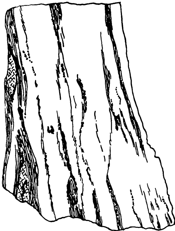
Fig. 5.—Ore from Blue Wing mine, showing banded structure. The white ground is calcite, with some quartz in little lenses. The solid black is bornite. The parallel lines represent schist. Scale, natural size. (After W. H. Weed.)
