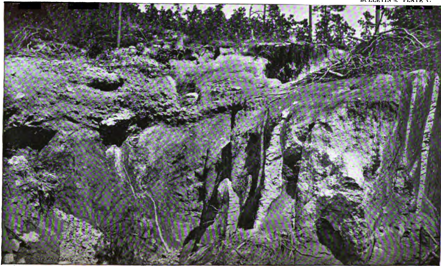
SMALL QUARTZ VEINS IN DECAYED SCHISTS, AND OVERLYING AURIFEROUS "GRAVEL."—SAM CHRISTIAN MINE.
