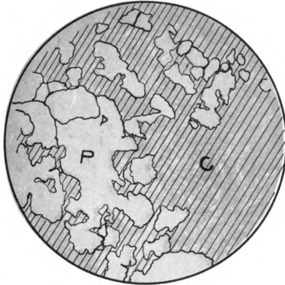
A—PHOTOMICROGRAPH SHOWING RELATION OF PYRITE TO CHALCOPYRITE. P—PYRITE. C—CHALCOPYRITE.
