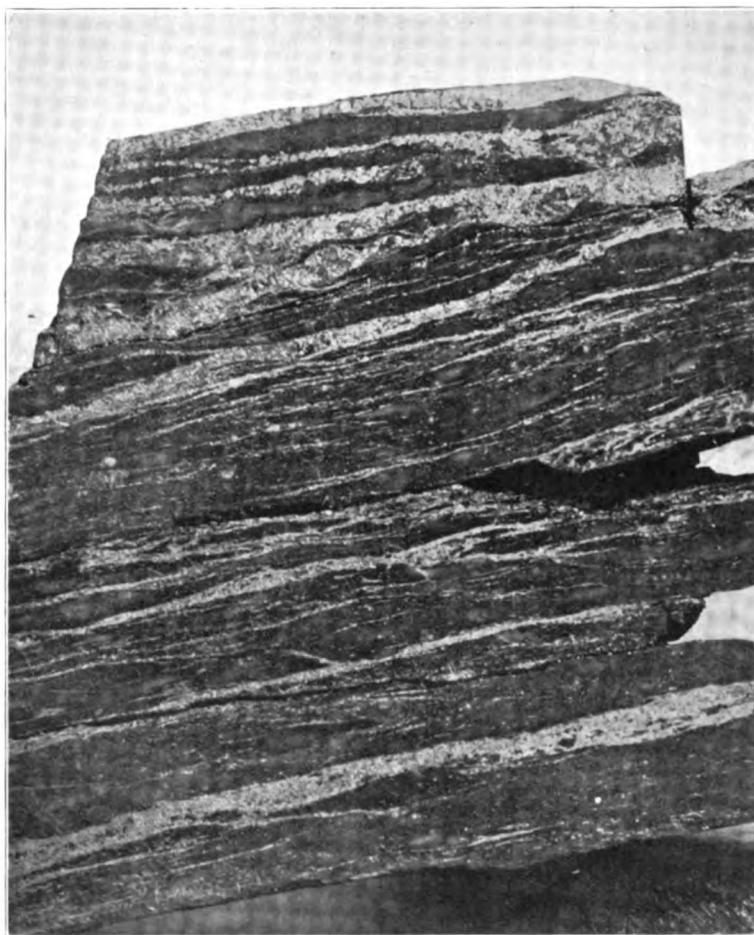
PHOTOGRAPH OF SMALL PORTION OF TYPICAL "SLATE VEIN," SHOWING ORE FILLING CREVICES IN RIFTED SCHIST. MILLER VEIN, GOLD HILL MINE. (Three-fourths natural size.)
