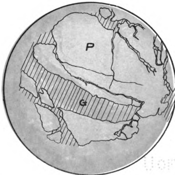
B—PHOTOMICROGRAPH SHOWING GOLD FILLING CRACKS IN PYRITE. G—GOLD. P PYRITE.
