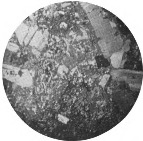
B. SAME IN POLARIZED LIGHT, SHOWING THAT MANY OF THE FRAGMENTS ARE OF ROCK SIMILAR TO THE GROUNDMASS. X 20.
