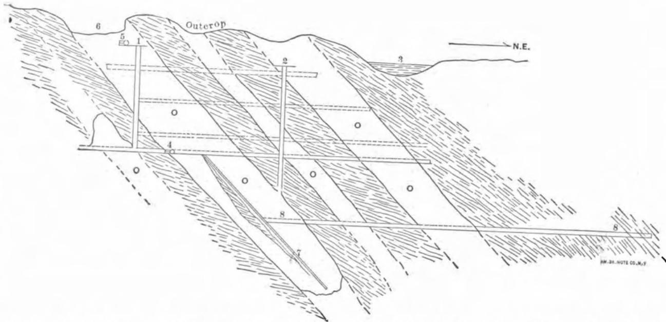
Fig. 20.—Vertical Section along the strike, Franklin Mine, Ga. Scale, 1 inch=200 feet. O, ore-bodies; 1, No. 2 shaft; 2, No. 1 shaft; 3, Etowah river; 4, underground hoisting engine; 5, surface hoisting engine; 6, Franklin Pit; 7, slope; 8, 350-foot level.
