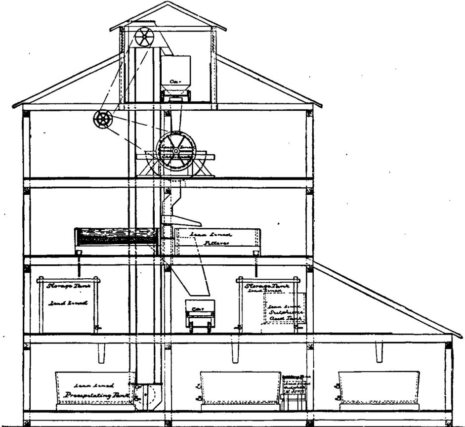
Fig. 29.—Chlorination Plant at the Halle Gold Mine. Vertical Cross-section.
