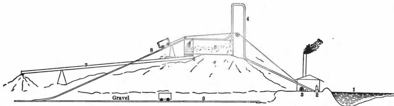
Fig. 6.—Sketch of method of working gravel at Crawford mine, Stanly county, N. C. (Not drawn to scale.) 1, reservoir; 2, pump; 3, holsting engine; 4, stand-pipe; 5, washing-box; 6, grizzly; 7, sluices; 8, inclined plane; 9, track on bedrock.
