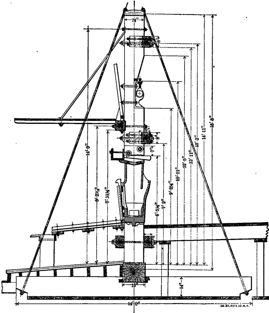
Fig. 16.—Vertical Cross-section of the 450-pound Hall Stamp-mill.
