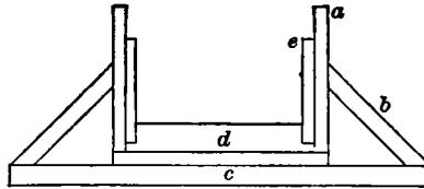
Fig. 12.—Section of Sluice-box, J. C. Mills land, Burke Co., N. C. Scale,  $\frac{1}{4}$  inch=1 foot. *a*,  $1\frac{1}{2}$ -inch surfaced pine plank (sides and bottom); *b*, 2x4-inch brace; *c*, 2x4-inch sill; *d*, 1x4-inch riffle; *e*, 1x8-inch sand-board.
