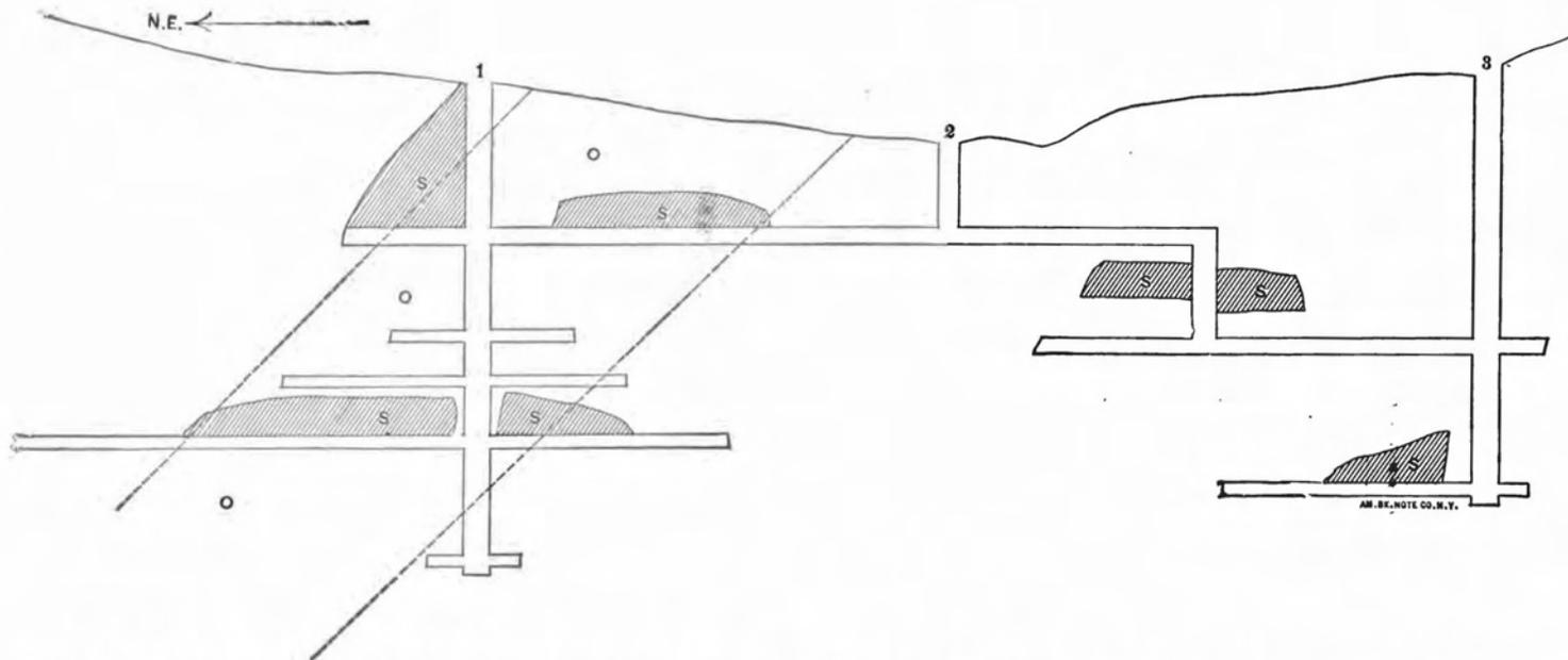
Fig. 18.--Vertical Section on the Strike of the Vein, Reimer Mine, N. C. Scale, 1 inch=80 feet. 1, shaft No. 1; 2, air-shaft; 3, shaft No. 2; O, dip of ore-shoots; S, stopped ground.
