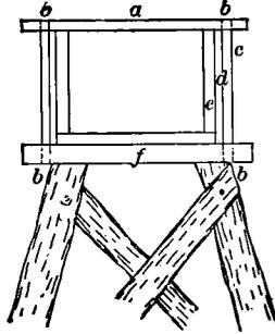
Fig. 10.—Flume, Mills Property, N. C. Scale,  $\frac{1}{8}$  inch=1 foot. *a*, 1x3-inch board; *b*, 1-inch holes; *c*, 1x3-inch board; *d*, wedging; *e*,  $1\frac{1}{2}$ -inch plank (sides and bottom); *f*, 2x4-inch sills and cap for bent.
