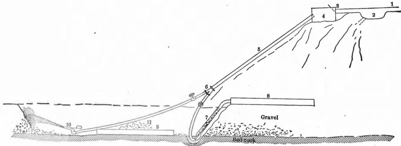
Fig. 9.—Sketch of proposed Hydraulic work on Mills Property, Burke County, N. C. (Not drawn to scale.) 1, ditch; 2, sand pit with drain; 3, screen at head of penstock; 4, penstock; 5, pipe (10 and 8-inch); 6, Y branching into two 7-inch pipes; 7, hydraulic elevator; 8, top sluice-boxes; 9, pit sluice-boxes; 10, giant; 11, boulder and pebble heaps.
