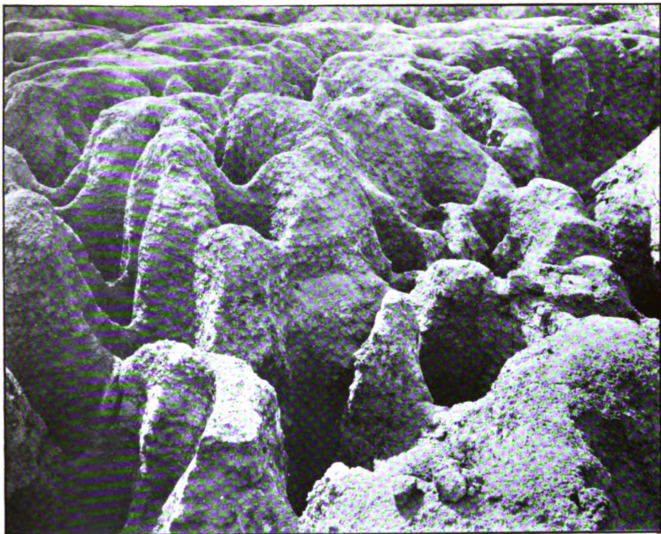
A. Marl beds, with overburden and sand removed, ready for steam shovel.—Trent River Marl Lime Company
