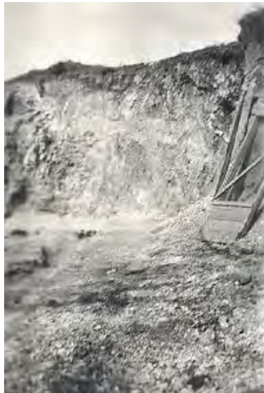
FIGURE 6 View of Kipps quarry with hand-screen leaning against quarry wall at right edge of photograph.
