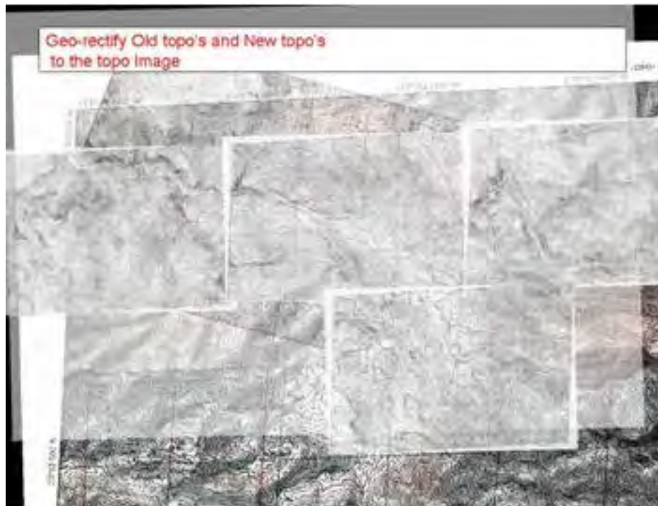
FIGURE 9 Stable base hard copies of original topography were georectified to current topography
