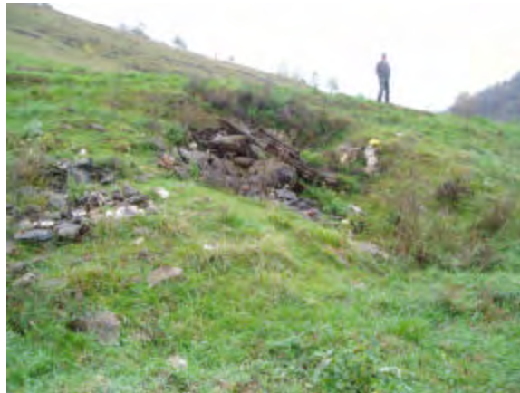
FIGURE 3a Primitive lime kiln, where rock is removed and replaced in quarried area with fuel and burned. After removal of lime, only a small quarry with traces of calcined lime-rock remain, seen under yellow GPS case. Waste partially calcined rock is visible on the mound in the left foreground.
