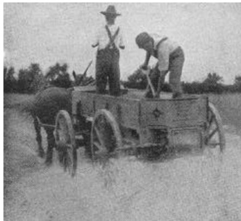
FIGURE 4 Illustration of an end-gate spreader in operation from old Stover Lime Pulverizer brochure. Note even distribution of lime, which obscures view of lower rear wheels. One person drove the team, while a second shoveled lime into the spreader unit, mounted on the wagon's end gate.
