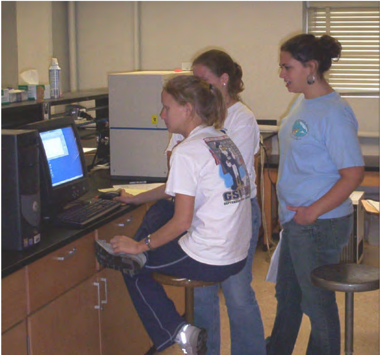
FIGURE 5 Undergraduates taking the Environmental Geology Laboratory course at Georgia Southern use JADE search/match software and a Rigaku Miniflex XRD unit to identify the mineral components in household products and construction materials.
