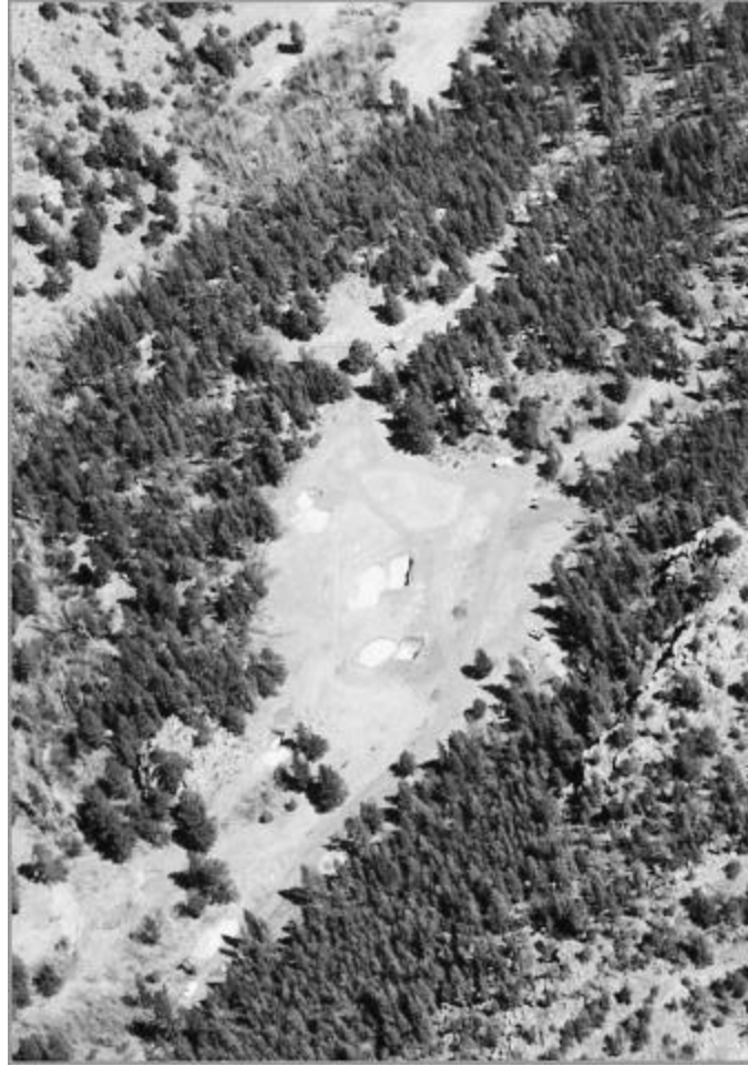
Figure 5 Aerial view of the Sloan 5 kimberlite, Colorado-Wyoming State Line district, showing distinct vegetation anomaly (high growth of grass and no trees) along a distinct lineament (photo by Hausel).
