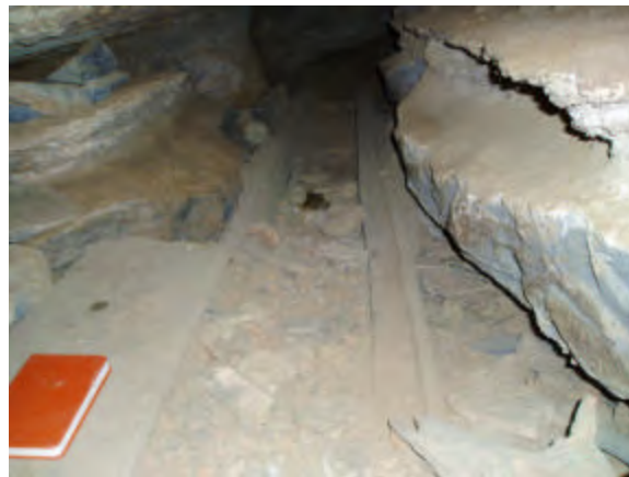
FIGURE 5 Wooden rail system used in Civil War era to haul nitrate-rich sediments through a project area salt peter cave.
