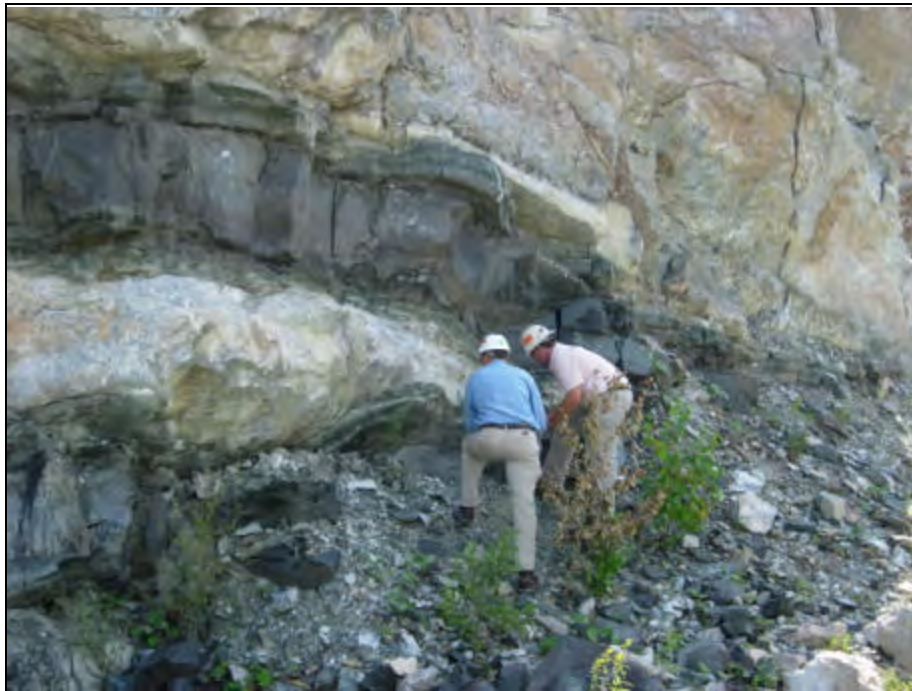
FIGURE 2 Mine personnel observe contact between the mafic lamprophyre dike swarm and the talc-magnesite ore.
