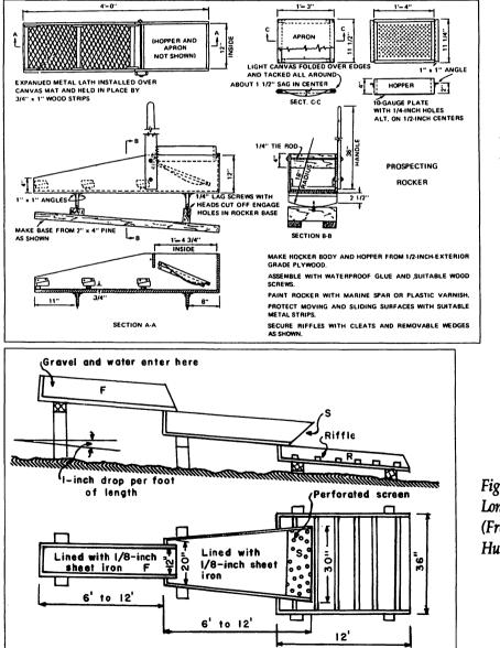
Figure 12. Prospecting rocker (From Wells, 1969).
