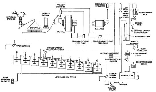
Figure 8. Flowsheet of Ridgeway mill and leach/carbon-in-leach facility, Ridgeway Mine, South Carolina. (Reprinted from Mining Engineering and published with permission.)
