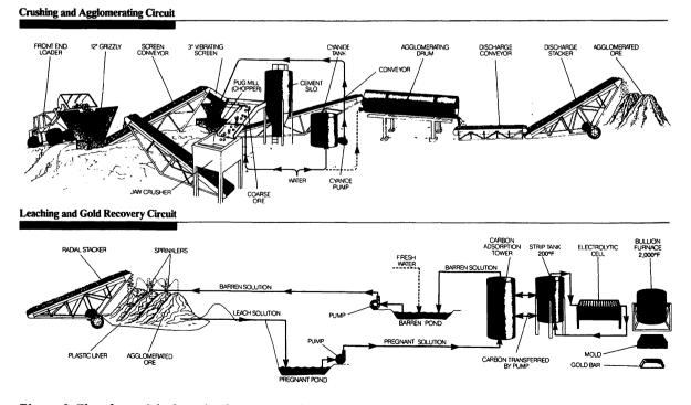
Figure 6. Flowchart of the heap-leach process at the Haile Mine, South Carolina. (Reprinted from Skillings' Mining Review and published with permission.)
