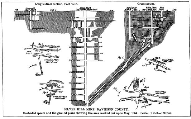
Figure 21. Underground workings at the Silver Hill Mine, 1854 (From Kerr and Hanna, 1893).
