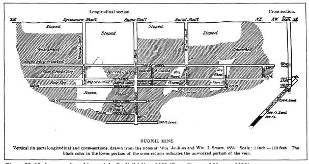
Figure 22. Underground workings of the Rudisil Mine, 1883 (From Kerr and Hanna, 1893).
