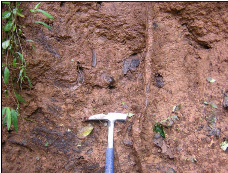
Figure 8. Close up view of decayed woody debris (dark areas) exposed in the August 22, 2005 debris flow head scarp at Site 2 (fig. 7). Hammer head is about 7 inches across.
