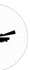
Unidirectional Rose Diagram of Joints N = 204 Outer Circle = 10% Mean vector = 92 degrees
