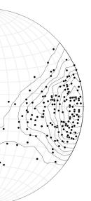
Equal-Area Schmidt Net Projection of Contoured Poles to Compositional and Gneissic Layering Contour Interval = 2 sigma N = 294
