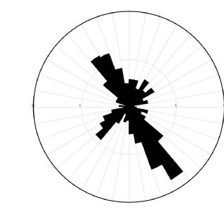
Unidirectional Rose Diagram of Joints N=488 Outer Circle = 10% Mean vector = 127° ± 43°;
