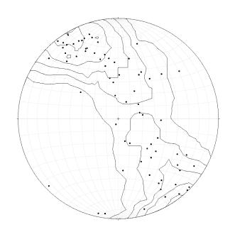
Equal Area Schmidt Net Projection of Contoured Poles to Primary Bedding and Layering Contour Interval =2 sigma; N=73
