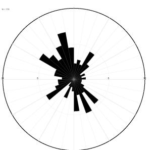
Unidirectional Rose Diagram of Joints N = 178 Outer Circle = 10% Mean vector = 337.1 degrees ± 14.9 degrees; Max value = 10.11236% between 151 degrees and 160 degrees
