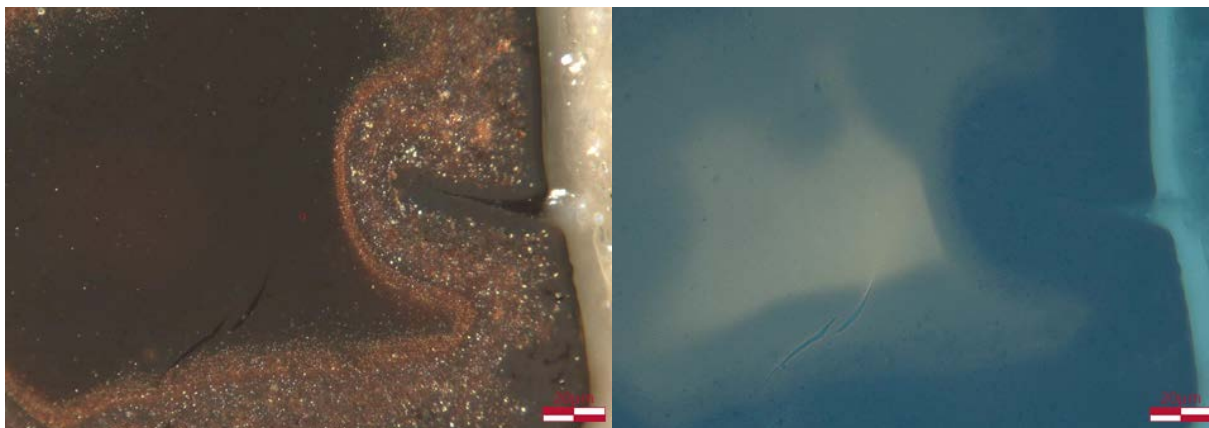
Figure 6. Esso #1 well Sample 6126527253 (7705'): (Left) Large particle of solid bitumen with desiccation cracks. Reflectance from central measuring circle is 0.19% Ro. (Right) Dull orange fluorescence from center of bitumen particle with distinct reductions in intensity moving towards perimeter (possible effects of biodegradation).
