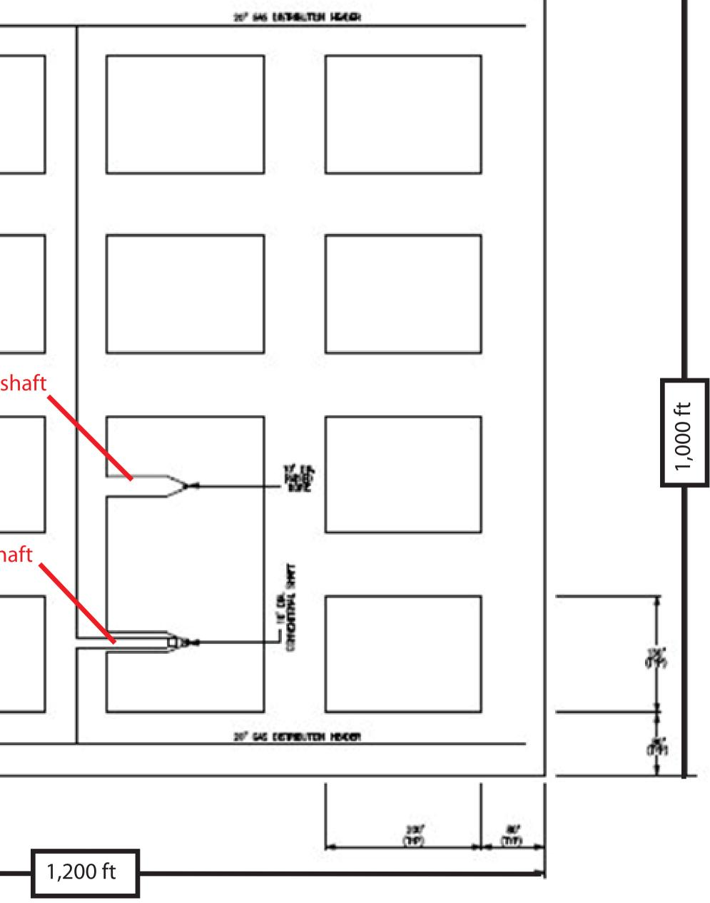
Plan view of a refrigerated mined storage cavern for natural gas. Layout at the 3,000 ft depth from PB-KBB (1998).
