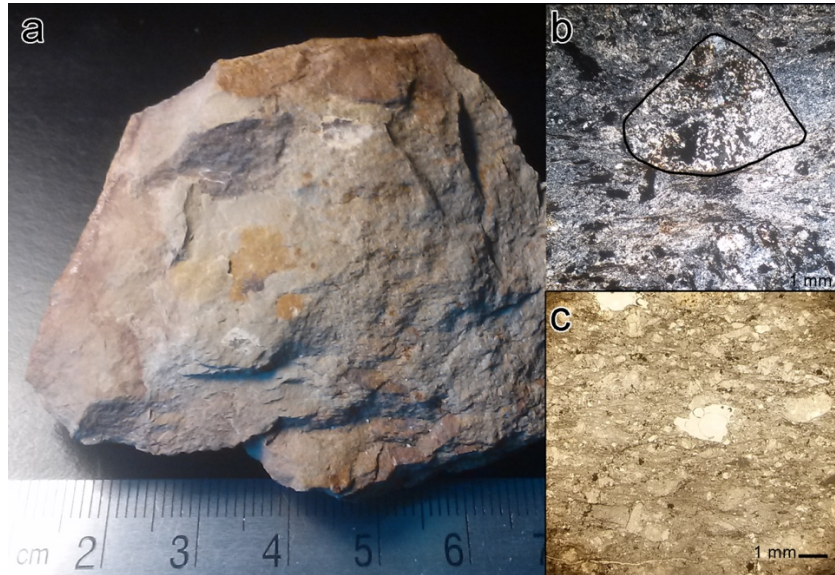
Figure 8: In hand sample (a) chloritic argillite is a dull grey-green with red to orange iron oxide deposits. In (b) at 100x with crossed polars, with a single clast centered in frame (outlined in black). Despite indistinct edges it can be identified by its coarser texture and disruption of the surrounding rock fabric defined by oriented chlorite crystals. In (c) at 40x with uncrossed polars the clastic nature of the rock becomes apparent, although almost all minerals have been largely chloritized.
