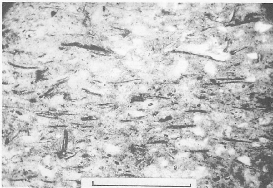
Figure 2. Photomicrograph of altered biotite flakes in Tioga Bentonite. Bar scale is 1 mm long.
