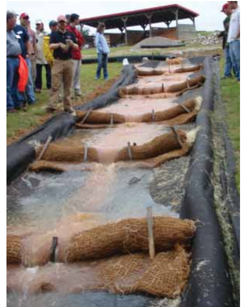
Figure 4. Polyacrylamide applied to fibrous check dams (FCDs) is demonstrated to treat runoff in ditch lines
