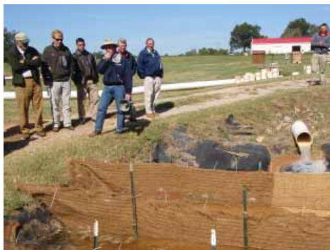
Figure 3. Dr. Rich McLaughlin explains the velocity reducing mechanism of coir baffles in sediment basins.
