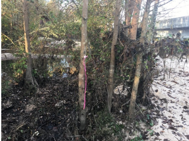
Photo of HWM 4 at Tree marked with nail, HWM disc and pink flagging approx. 30 FT from Dunn Rd. at start of tree line. Cumberland County, NC, 10/20/2016. Photograph by Chris Brown, USGS GA.
