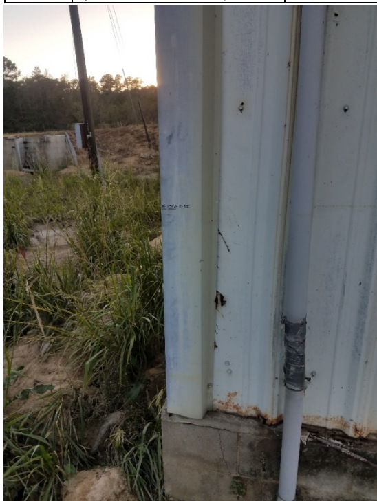
Photo of HWM2: On side of Houses mill. Marked with sharpie, Sampson County, NC, 10/23/2016. Photograph by Chris Brown, USGS GA.
