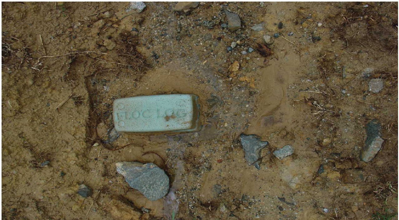
Flocculants are used to pull the finer particles out of the water to reduce turbidity, and protect sensitive water resources.
