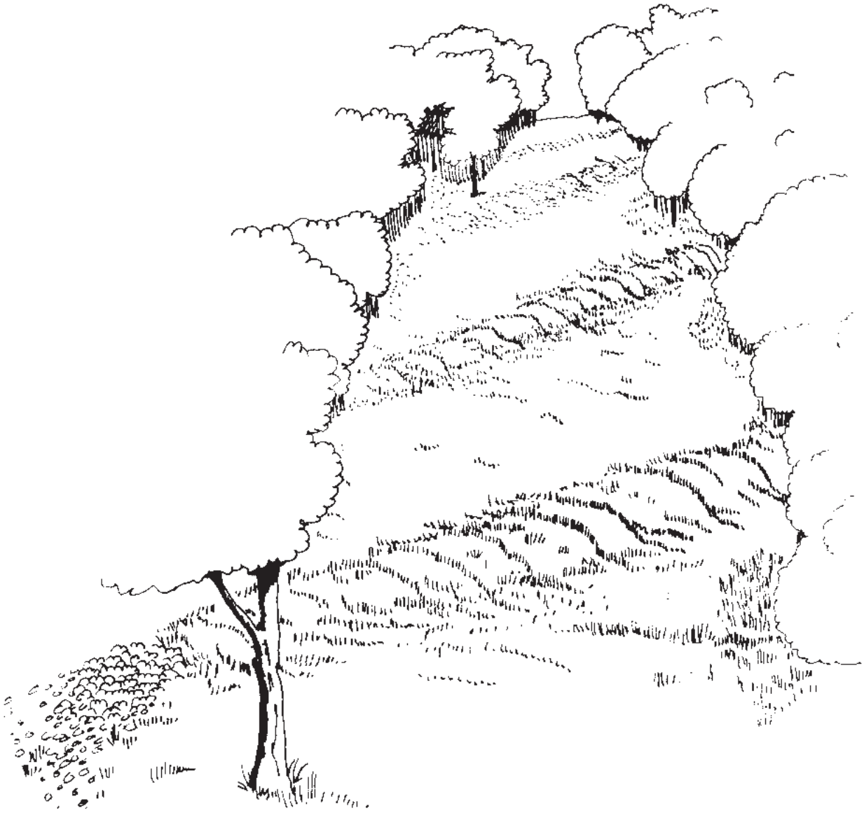
Figure 6.23a Water bars to protect utility right-of-way.
