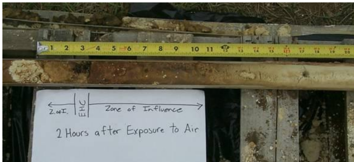
Figure 7: Photograph of a soil core, from 30 ft to 33 ft bgs, showing a 1-inch EHC seam.
