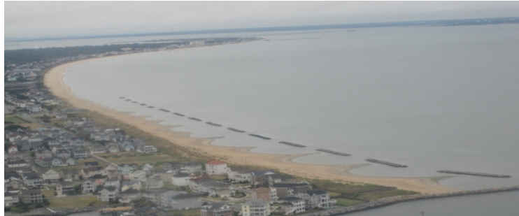
Series of breakwaters showing "tombolo" effect
