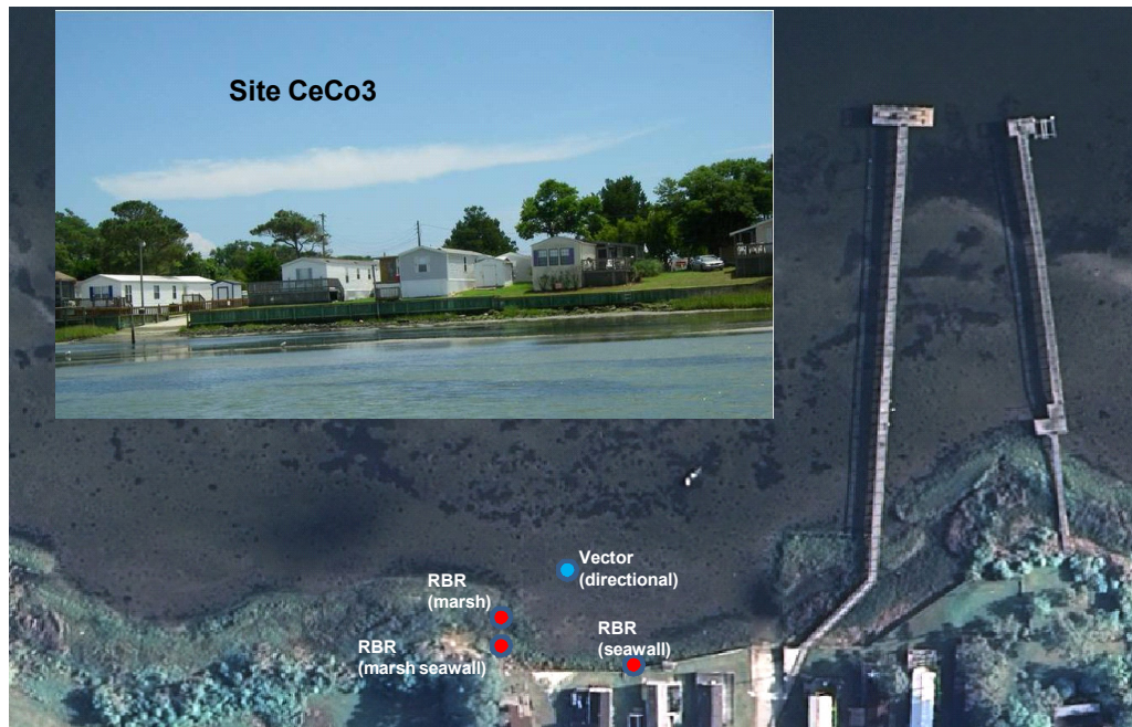
Figure 3: Wave sensor deployment at CeCo site. Directional wave information is provided by the Nortek Vector (blue dot). RBR pressure sensors measured wave energy in the marsh, at the foot of the seawall, and at the foot of the seawall in the marsh.
