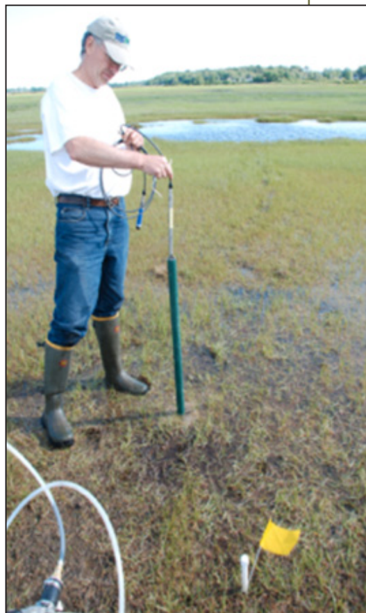
Deep groundwater monitoring well with Aquatroll 200™ data logger
