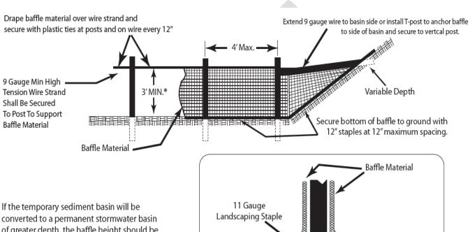
\* If the temporary sediment basin will be of greater depth, the baffle height should be based on the pool depth during use as a temporary sediment basin.
