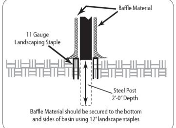
Figure 6.65b Coir Fiber Baffle Detail Cross section of a baffle in a sediment basin.
