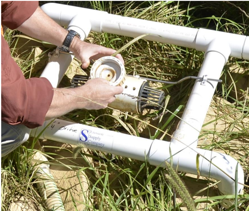
Orifice plate within union joint on ECS skimmer
