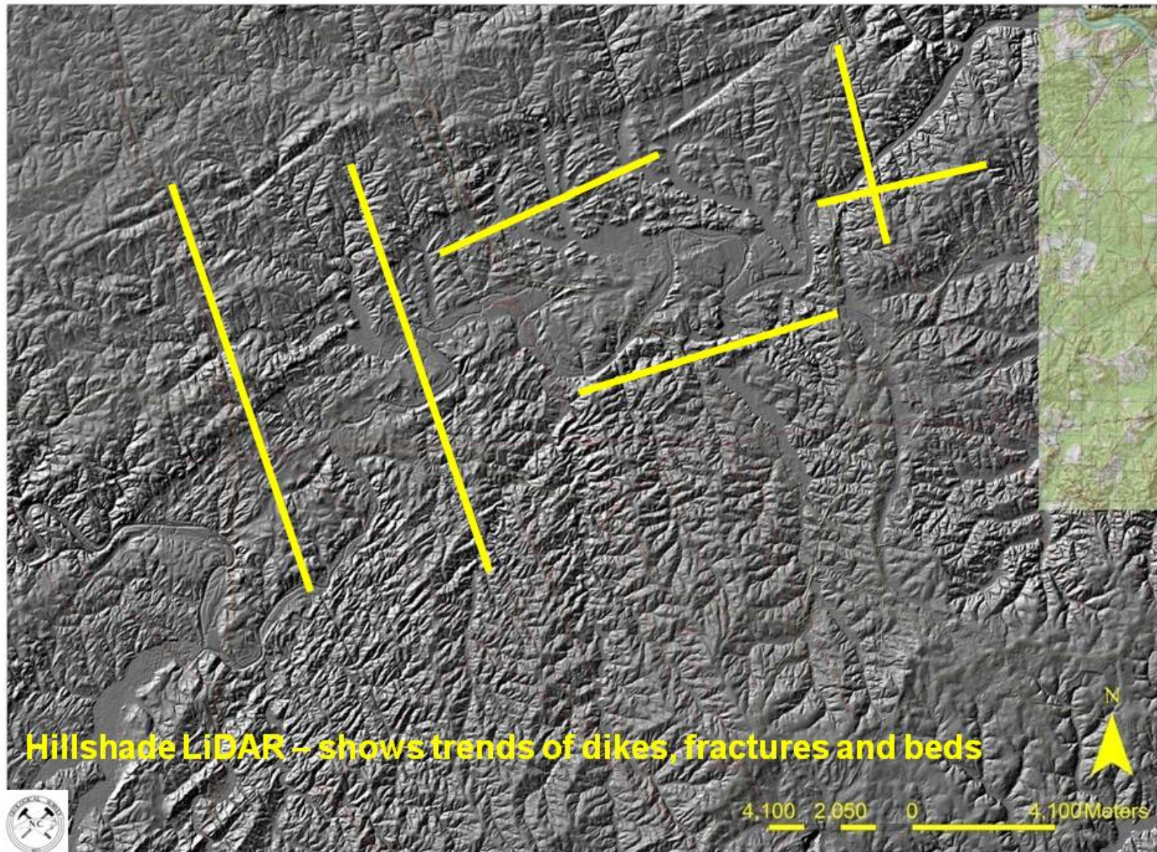
Figure 8. Hillshade LiDAR shows trends of diabase dikes, fractures and trend of sedimentary strata. The Deep River forms a sinuous border between Lee and Chatham counties, NC. The Sanford sub-basin occupies low relief terrane in the center of the image. Diabase dikes trend along northwest-striking fractures. The orthogonal fracture pattern observed in this image can be found at the outcrop scale and will be of interest to natural gas exploration and production.
