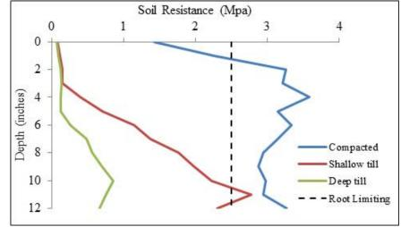
Figure 5. Soil resistance, a measurement of compaction, measurements made using a penetrometer at the Raleigh, NC sit. Clay soil at field capacity.
