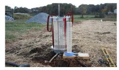
Figure 1. Cornell Sprinkle Infiltrometer used to make infiltration measurements.
