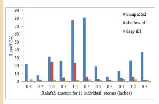
Figure 7. Percent runoff for three tillage depths (none, shallow, deep), for 11 storms at the Raleigh, NC site. Rainfall values indicated below each storm. Deep tillage produced less than 2% runoff for all storms, compacted sites generated the most runoff for all storms.
