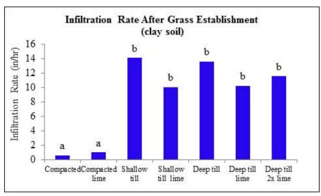
Figure 6: Infiltration rate measured with a Cornell Sprinkle Infiltrometer at the Raleigh, NC site. Collected after grass had established and some soil settling (tilled). Different letters above means correspond to significant differences at P = 0.05.
