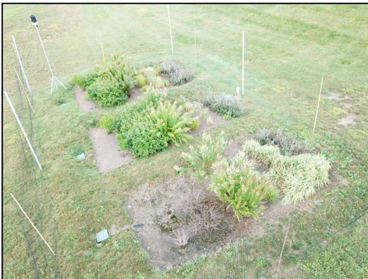
Aerial view of the soil blend study showing the three bioretention cells, with the standard practice in the foreground with the dead plants. Photo credit: James Funai.
