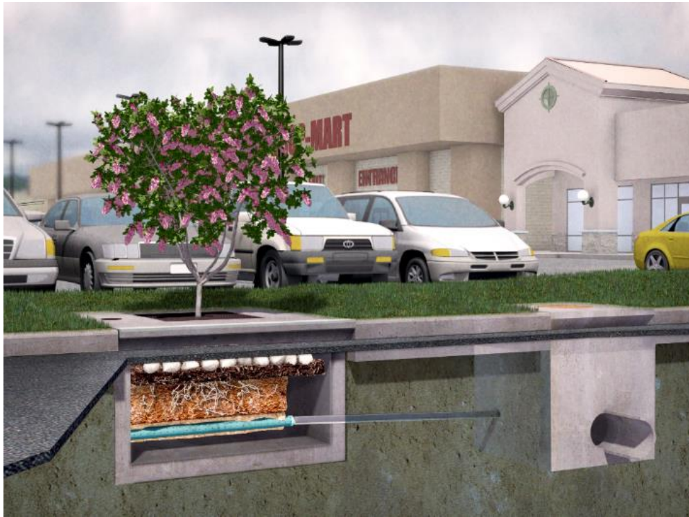
Figure 1: Filterra Offline Configuration
