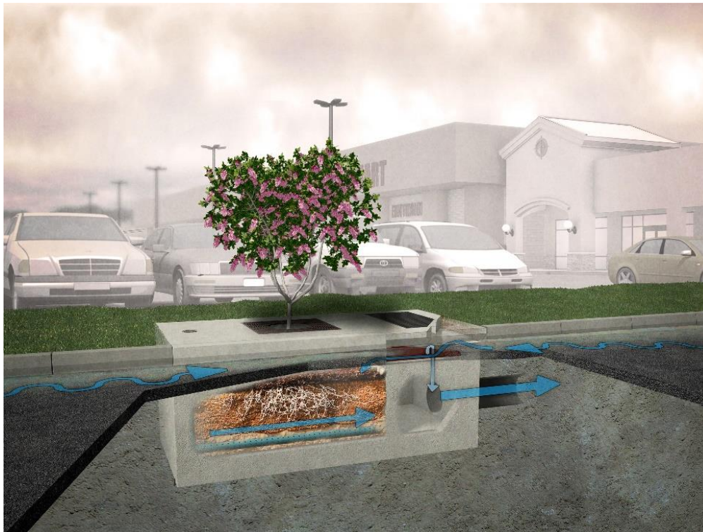
Figure 2: Filterra Internal Bypass Configuration
