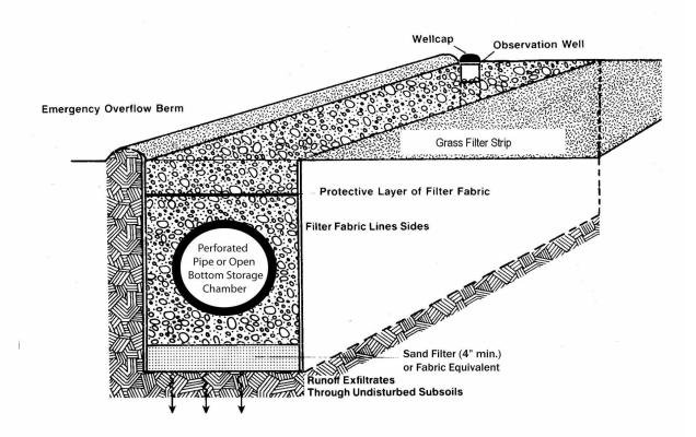
**Figure 16-1b** Typical Infiltration Trench: Cross-Section
