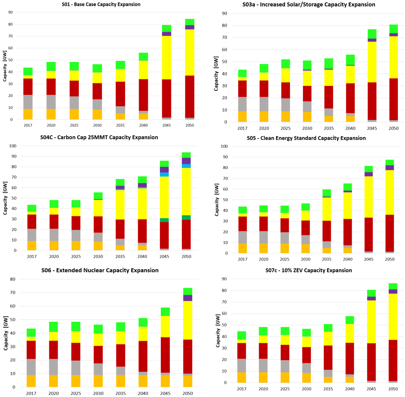
Figure A. Installed generation capacity in gigawatts (GW) through 2050 corresponding to the generation results presented in Figure 1. Note that the Duke territory is modeled, and generation results are scaled to reflect the proportion of generation in North Carolina.
