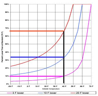
Effect of Lowering Thermostat Setpoint On Heat Loss
