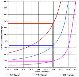
pump power, and control regulation power) of 21,200 kWh @ \$0.086/kwh = \$1,823. Additionally, natural gas consumption was 1,950 therms at \$1.16 /therm or \$2,262. The total heating bill for the month would be \$3,174. Based upon an average temperature of 40 °F what is the cost savings for a 3 °F, 10 °F, and 20 °F setback at night. Since the unoccupied portion of the day is 14 hours in 24 hours or 58 % of the heat loss should be allocated to the nighttime setback energy use or
