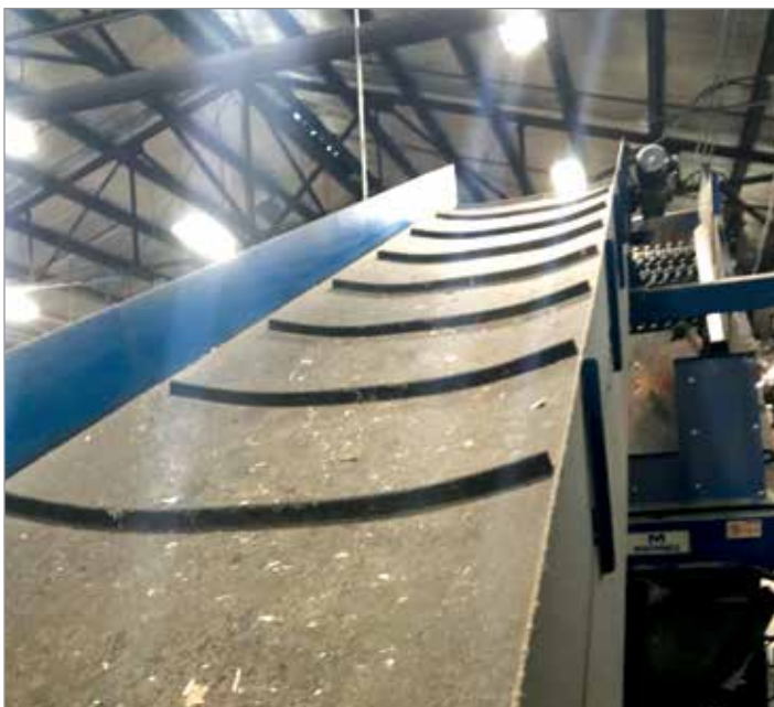
American Recycling leveraged grant money from the state of North Carolina and the Glass Packaging Institute to replace its glass breaker and make other system improvements at its materials recovery facility.
