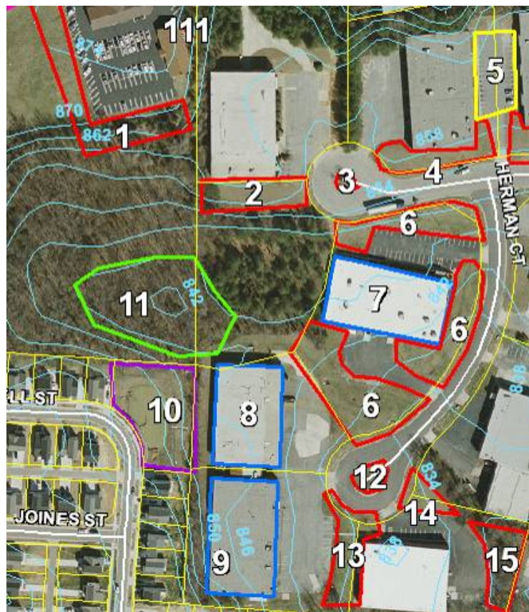
Figure 2. Potential stormwater control measure (SCM) retrofit sites identified via GIS analyses (red shapes indicate a potential bioretention SCM, yellow indicates permeable pavement, green indicates a wetland, purple indicates an existing wet pond, and blue indicates a potential water harvesting opportunity).
