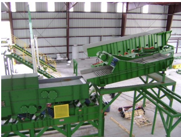
The two-stage screeners are designed to maximize the recovery of recyclable materials from the mixed C&D material stream.
