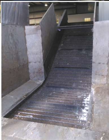
The conveyor and compactor shown here in GBUSA's spoke model were designed to fit into a compact area and have proven effective in consolidating commingled recyclables for transport to market.
