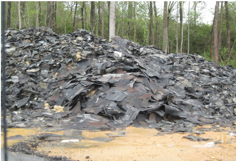
Clean piles of tear-off asphalt shingles from Harnett County rooftops await processing at the Johnson Brothers Utility and Paving Asphalt plant.
