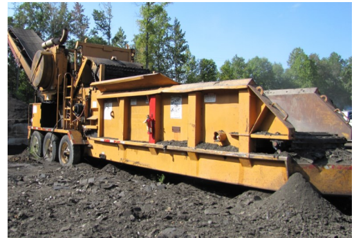
A grinder processes shingles to the size of coffee grounds.
