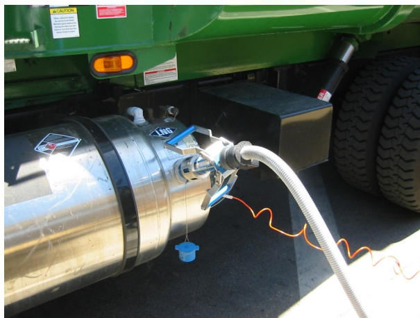
A waste collection truck, shown above, is filled at a fast-fill CNG station, much the same as a traditional gasoline filling station.
