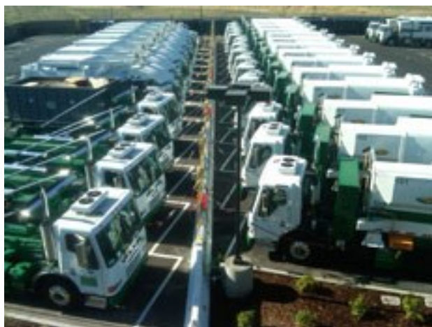
Waste collection trucks shown above are being refueled at a time-fill CNG station.
