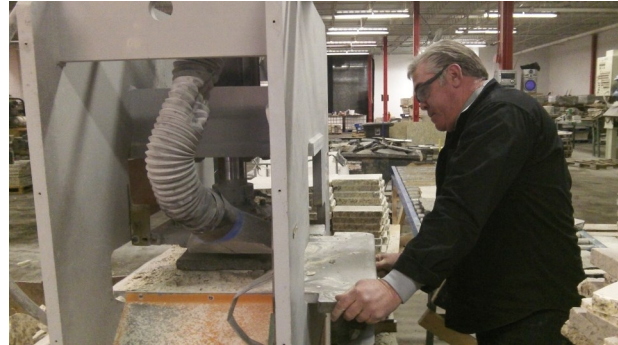
EarthStone's Sandy Brady stamps out a recycled patio paver from granite countertop scrap.
