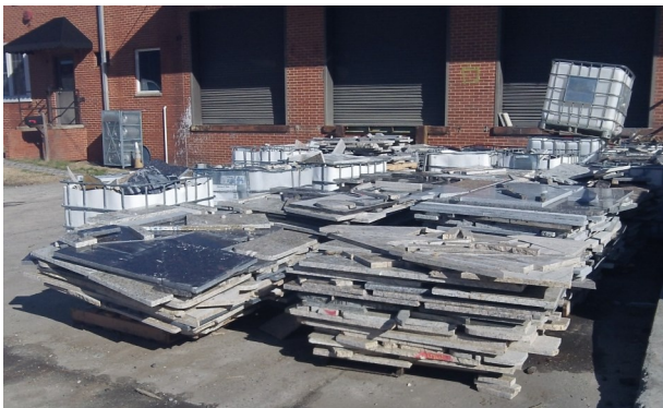
Granite scrap from countertop installations are received at EarthStone for transformation into granite patio pavers and other granite tile products.
